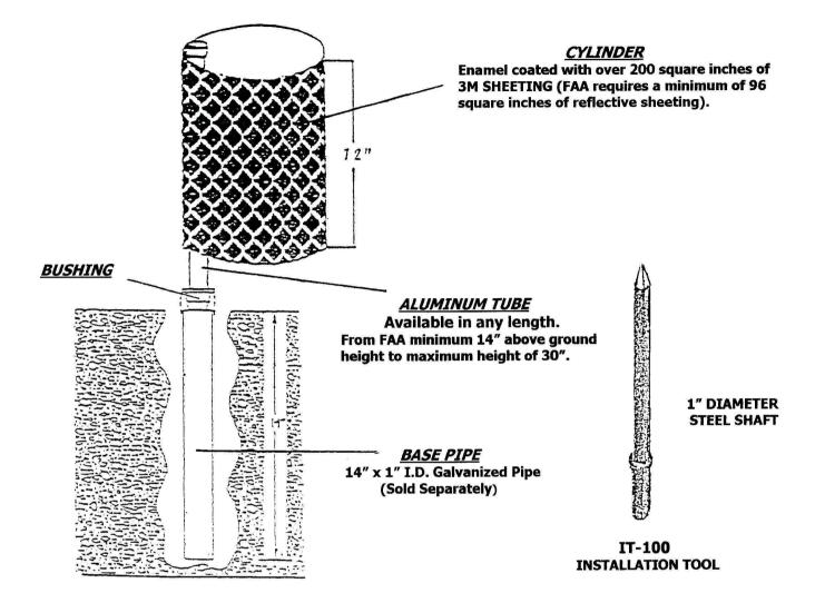
THE BASE PIPE IS EASILY INSTALLED, USING THE IT-100 INSTALLATION TOOL. MOST SURFACES CAN BE EASILY PENETRATED USING THE IT-100 IN A JACK HAMMER. SIMPLY INSERT THE TOOL IN THE BASE PIPE AND DRIVE THEM BOTH INTO THE GROUND AT THE SAME TIME. REMOVE THE INSTALLATION TOOL AND PUT ASSEMBLED ILLUMINATOR AND BUSHING IN BASE PIPE.
